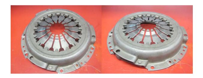
Examples of a "FLAT FINGERED" pressure plate that should not be used the HVDA conversion.
