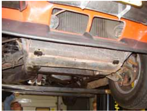
VIEW WITH OLD SWAY BAR REMOVED
