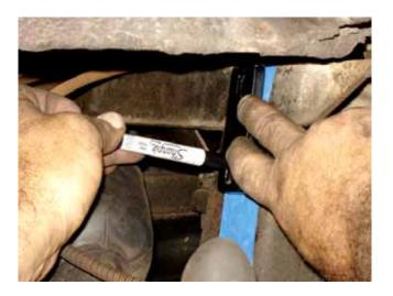
4. Remove the bracket and center punch the holes. Using your right angle drill adapter and the stubby drill bit, drill the holes through the tower support. Remove any chips form the back of the holes. Perform the same procedure on the other side.
