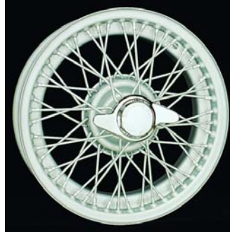
A 48-Spoke Painted Wire Wheel as Fitted to TR-3 Models (Dayton Wire Wheels)
