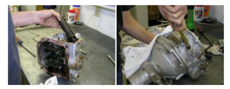
The early overdrives (models 22/1374 and 22/1712) have a large accumulator and piston. The piston has threads that are 3/8x24 so it can be removed by prying on the head of a long bolt screwed into the piston.
