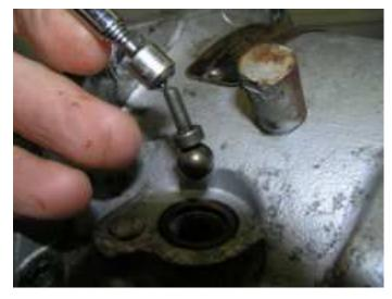
You can check the operation of the unit by reinstalling the ball, applying air pressure at the plug hole and manually activating the operating valve. The operating pistons should move the sliding assembly forward until the brake ring is contacted.
