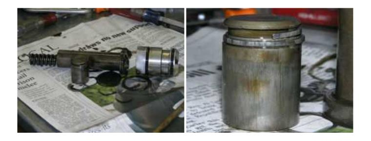
**Step 6 – Remove the Operating Pistons**
