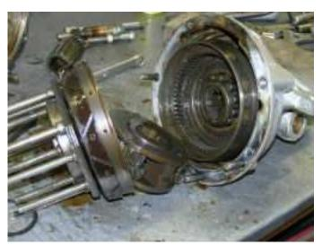
expensive. If it rolls smoothly, you may wish to reuse it. If you replace the bearing, you must remove the snap ring (circlip) that secures the thrust ring to the sliding member and the snap ring which holds the bearing.
