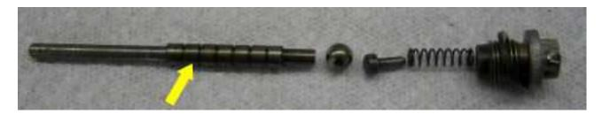
Step 5 – Remove the Accumulator Piston
