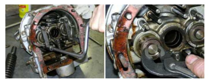
The left photo shows the early style piston with steel rings (model 22/1374), while the right photo shows the later style with rubber o-rings (models 22/1712, 22/1753 and 22/1985).
