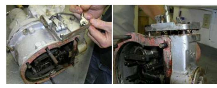
Once the plate is off and the springs withdrawn, the piston can be removed. Air pressure can be used to move the piston. Temporarily reinstall the ball in the operating valve, then (see photo) apply pressure at the operating valve plug hole. This initial movement can help to dislodge a stubborn piston. Sometimes air pressure will blow it completely out, so use a towel to catch it. You can now remove the operating valve.
