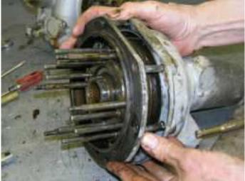
The picture to the right shows the housing for our bodged TR4 overdrive. The flange of the main housing was broken off and the housing itself was cracked. We suspect the overdrive was dropped. The grease in the broken area indicates it may have been put together this way. Since this is a valuable piece, we had it repaired at a machine shop.
