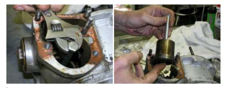
The later overdrives (models 22/1753 and 22/1985) with small accumulator have a sleeve and spacer tube in addition to the piston. If air pressure does not remove all three pieces, you can make an extraction tool using a rubber expansion plug (like a drain plug for a boat). A good hardware store will stock rubber expansion plugs in a variety of sizes.
