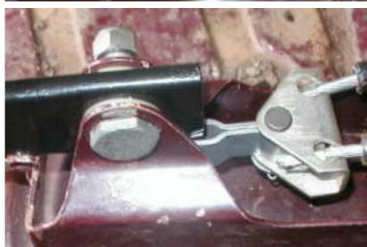
The outer cables were then slid over the notches in the bracket. If there is insufficient cable slack, the pins attaching the fork end to the rear wheel cylinder lever can be removed and then reinstalled after the outer cable has been positioned.
