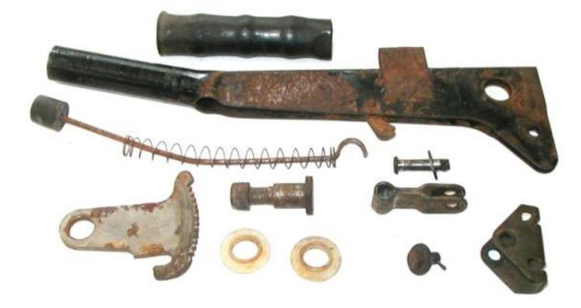
Some of these parts are obviously in worse shape than those of the '76 handle. For example, the '70 paw release knob has a hole as shown on the right. Won't speculate as to why handbrake was applied with such urgency to make the hole. I decided to use any part from the later lever assembly that was the same as for the early lever assembly and in better shape. (I also have a '76 so wanted to keep the unique '76 parts.)
