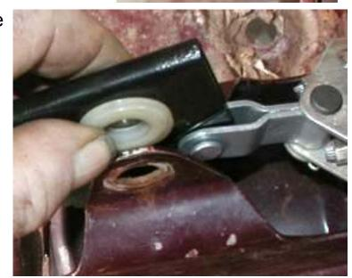
The ratchet segment is then aligned so that the shoulder on the fulcrum bolt will slide through the bracket, the nylon bushes and the ratchet segment. Probably the best tool to use is a tapered drift (punch). I forgot to take a punch to the shed for this photo shoot so the screwdriver was used and turned out to be a poor substitute.
