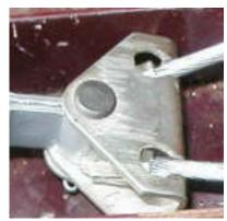
The ratchet segment is then hooked over the front tab of the handbrake bracket
