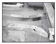
away. Installing new trailing arm mounting repair sections will pretty well dictate that you install new upper & lower cruciform plates as well. They will be ruined during the removal process.
