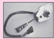
switch is correct for all 75 - 79 cars. Works just fine on 80-81 cars too. (The only difference being the shape of the plastic on the end of the lever.
