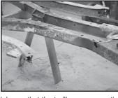
you can plainly see that the trailing arm mounting "legs" have completely broken away. This has left gaping holes where these frame sections once
