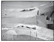
chassis rails are almost totally rusted out. The strength of this frame is badly compromised. Repairing the rusted out frame rails is easy when the damage is open and fully exposed. New steel plates can be grafted into the main rails and then new upper & lower cruciform plates installed.
