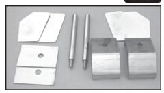
Engine torque pulls hard on the RH front differential mount. A car that has been driven hard (like popping the clutch and burning rubber) will more likely have damaged differential mounts. The differential hangs on steel pins that are welded into the chassis frame rear cross member(s)
