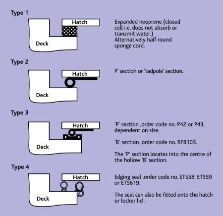
Please note that there are many different styles of hatches. The above drawings have been simplified to clarify the seal designs. Seals can either be fitted to the hatch, deck or both. Generally it is better to fit it to the hatch as it will help prevent it from being damaged or dislodged.
