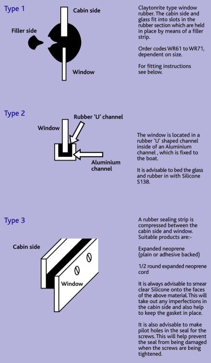
Note:- We also recommend the use of a sealant (order codes S136 to S138) under the heads of fixing bolts to help prevent water penetration.
