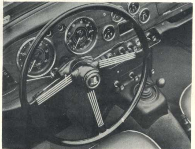
On this left-hand drive TR4A the new lighting control lever is on the right of the steering column (on the left of the right-hand drive version). Note also the recessed switches on the central panel.
