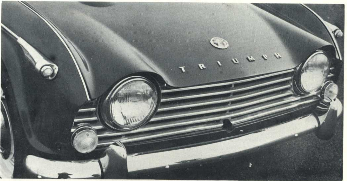
A sleek new grille, overriders set further outboard, chromium side flashes and the Triumph "world" motif, distinguish the TR4A from its forerunners.
