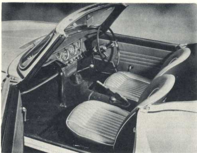
Fully carpeted and with padded and trimmed waist rails, etc., the Spitfire also has more comfortable seating.
