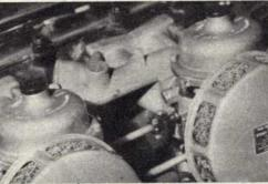
TWIN STROMBERG carburetters (type 175CD) are used in place of the S.U. in later versions. These carburetters can be obtained as a conversion kit at an exchange price of £18 from the Zenith Co. Ltd. They are claimed to provide both better performance and economy
