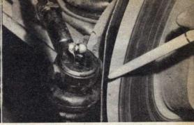
TRACK ROD ball-joints should not in any circumstances be over-greased. Over zealousness will permit grease to escape past the rubber boots and affect braking efficiency as the excess grease will be blown back on to the disc at high speed. Wipe away any excess lubricant
