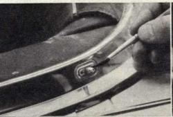
CHROME SCREWS holding the hood clips cannot be fitted without a risk of nicking the chrome surface and, if this occurs, the result after a time could be that the screws will rust. There is a simple means of preventing this. Apply lacquer or wax polish to the screws
