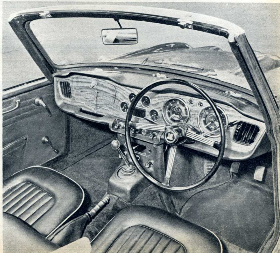
New handbrake location between the seats increases the effective width of the driving compartment, and the walnut instrument panel will appeal to many buyers
