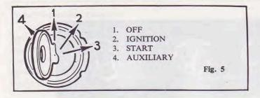
position the key may be withdrawn ; 2, "Ignition" ; 3, Start ; 4, Auxiliary. (See Fig. 5.)
