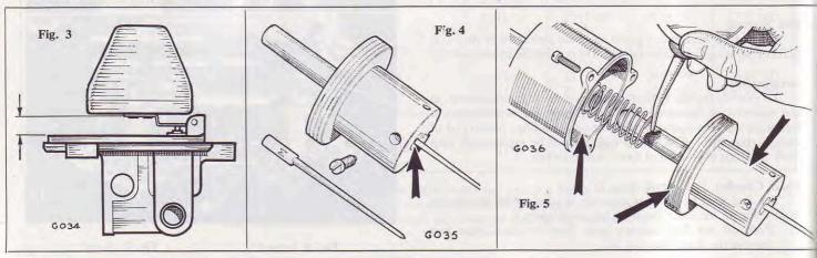
The needle size is engraved on the shoulder of the needle, which should be fitted with the shoulder flush with the under face of the piston and retained by tightening the screw.
