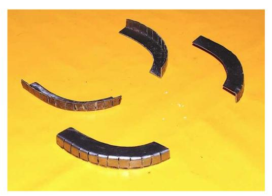
The hooks for the diaphragm had worn the rails of the drivers seat almost through to the edge of the rail! These required welding up and re-drilling. If I were doing this again I'd drill them outer bigger because I found filling a 1/8in slot with weld to be quite tricky.
