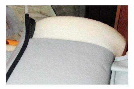
Wadding adds the curvature required and is cheap and obliging stuff to work with.
