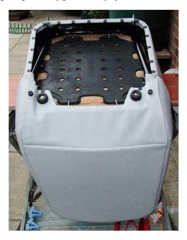
Note the use of a small screw and washer to trap the end of the top-cover. Originally this was done with a ring-clip around the frame-tube. The reinforcing plate are in the way for this to work and the leather is a bit too thick for them to hold properly.
