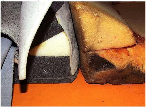
The foam seems to lean "the wrong way" but it won't do this when the cover pulls it. The white wedges are about 1in thick at this point.
