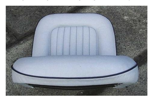
A bit of extra wadding was stuffed in here to get the right finish. Remember that these seats are not symmetrical in this area, so what works on one side does not necessarily work on the other.
