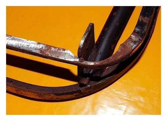
I used 10mm angle from my local hardware store on the front and sides. At the corners I made round repair pieces using 1.2 mm sheet folded and gusseted so it would form round a curve. I left the original corners pieces in situ and welded the repair pieces to them.
