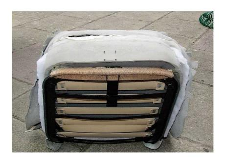
I added a loop of self-adhesive foam tape, 1/4in thick, to the frame and this can just be seen above. It runs under the Hessian and right down both sides.
