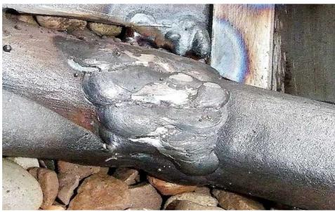
Whenever I weld a crack, in a place subjected to cyclic loading, I always add something to try to stop another crack forming. Remember that a weld upsets the carbon/iron balance in the steel and this means harder areas meet with soft areas along the weld line. This makes welded repairs likely to fail again.
