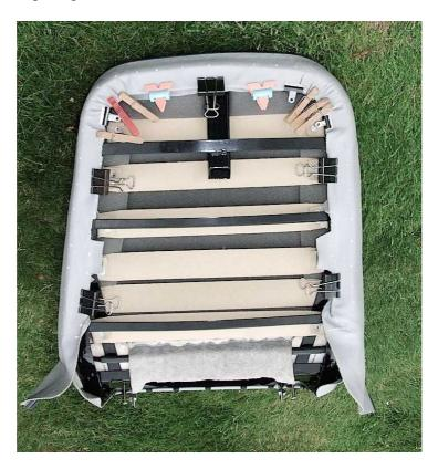
Now you have the **strenuous** task of installing the long spring that holds the bottom of the back-cover. This threads through the tube sewn into the cover and hooks into the lowest holes in the frame.
