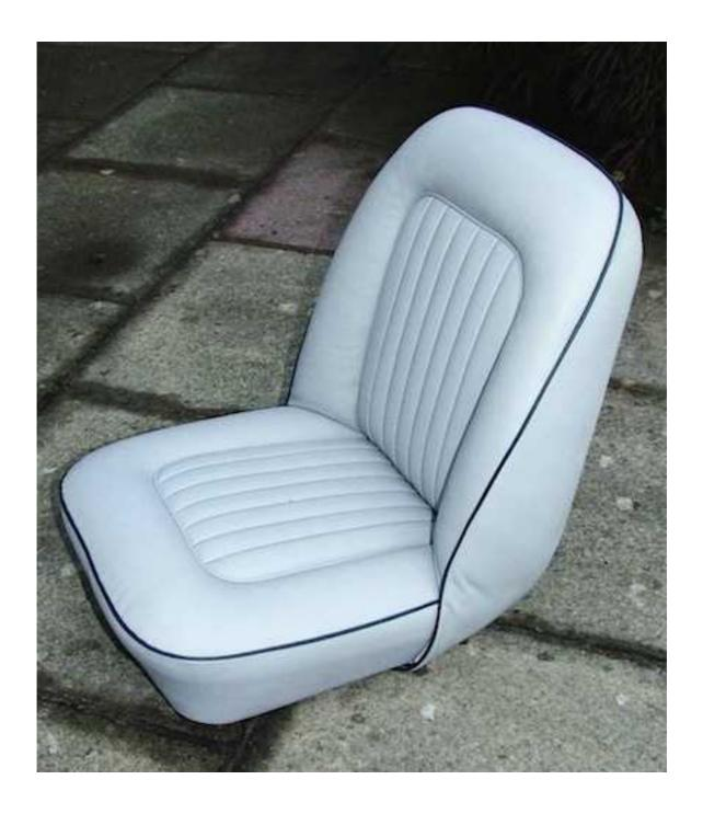
At this stage I still have not worked out how to secure the bottom corners of the cover for the seat-back. Leather is not compatible with the round clips used for Vinyl at this position, its too thick.
