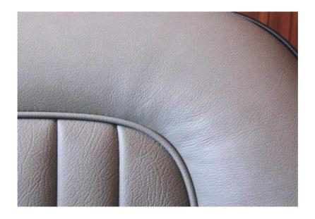
The two pads were made from offcuts of the hardest white foam, bought to make the head-rests. They were roughly shaped using scissors and scalpel and finished with the grinder.
