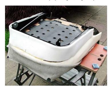
The frame can now be squashed down to its final position and the leather-cover drawn over the skirt and clipped temporarily in place.
