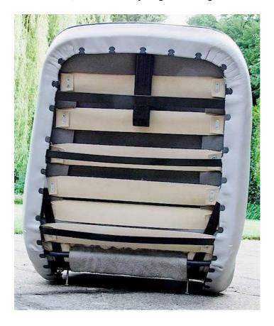
The small rubber feet were added so that I could put the seat down after the big rubber feet were fitted in place of the long screws. The big feet dont touch the ground!
