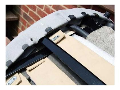
The small rubber feet also provide a means of securing the "flap" on the rear-panel to the curved part of the frame. Its also held by the big feet and some U-clips.
