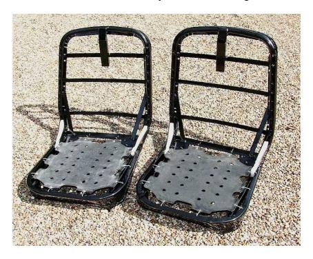
You can see that I have filled the gap between the two re-inforcing plates with white foam. Its actually closed-cell polyethythene foam recovered from packaging.
