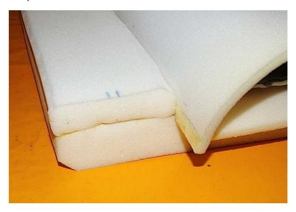
You can easily alter the shape of foam using rough trimming with a scalpel or electric carving-knife. You finish smooth with an **angle-grinder** with and ordinary steel grinding-disc, **yes really**!
