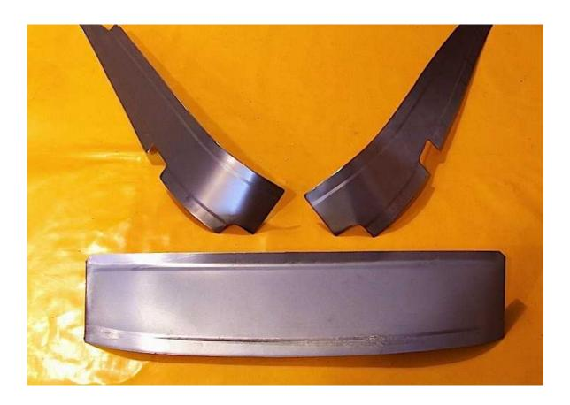
Note the cut-out that goes around the old strap that joines the two rails together. I retained this strap just to keep the whole thing in its original alignment.
