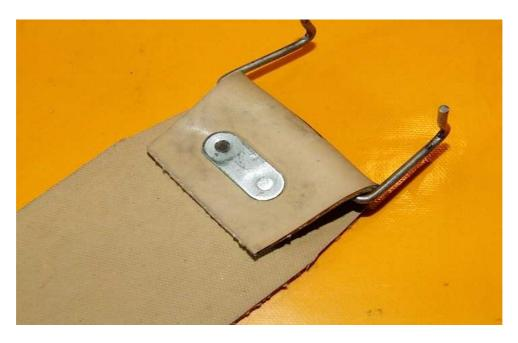
Its not hard to drill out the rivets and recover the fish-plates. I was fortunate that a "Model Engineering" supplier nearby stocked the right kind of rivet. And I had the rivet-snap to set them.
