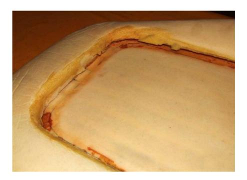
I prepared the new foam to accept the seam, by making a cut into it, about 1/4in deep. The cut went at an angle of about 5-10° below the glue layer, rather than following it or going straight down into the base layer. I had also added a layer of foam and this also helped to form a pocket to bond into. The leather seams are stiffer than Vinyl and this angle conforms with their "natural" lay.
