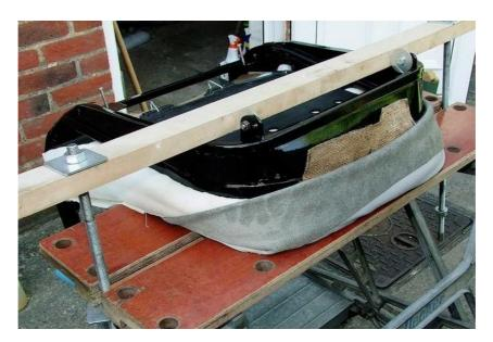
Here its about half-way into the final position. At this point check that the foam is correctly positioned both fore-and-aft and side-to-side, glue the Hessian flap to the front of the frame and clip the other flap around the rear cross-bar.
