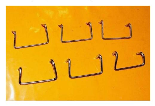
These clips were originally held into the ends of the straps by rivets passing through two oblong fish-plates. The modern replacement for this is a "staple" and these are easily available from suppliers of the Pirelli-webbing.
