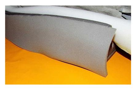
You can choose to use brush-on high-temperature impact-adhesive or the quick and easy spray-can stuff. Do not expect the can to generate anything like the joint strength of the brush-on kind.
