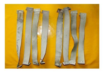
I set up a test with some new webbing by trapping a 1m length under my kitchen door and making marks on the floor to show how much I could stretch it. I could **easily** pull a 5% increase but to get 10% took a determined show of strength.
