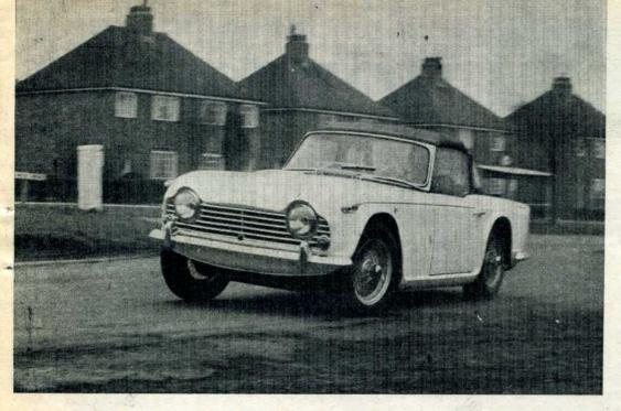
TR4 A displays new six-bar grille, side indi-cator lights mounted high on front guard. These are sup-plemented by plemented by parking lights in the grille. Left windscreen wiper has crooked arm to give better sweep. Hood is easily folded in one movement. Interior is improved, as is handling.
