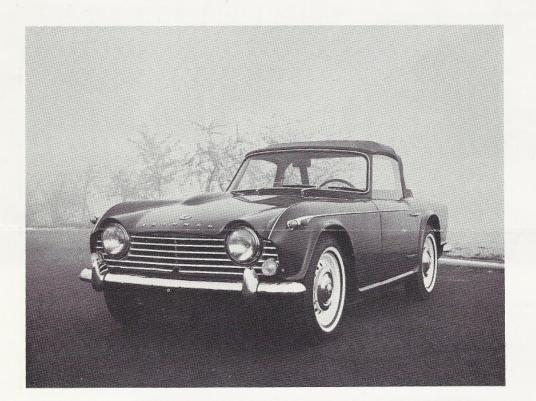
Photo on the left shows the new grille treatment on the TR-4A—latest model in the TR range — which gives a cleaner, more horizontal appearance to the front end. Also clearly visible are the re-positioned flashers — now mounted on the front fenders and easily seen both from the front and side of the car. The new top is up in this shot ...
